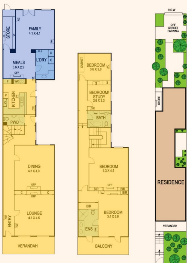
Figure 2 Façade (top) and plan (bottom) of 51 Drummond St showing original areas to be reproduced (yellow) and new extensions to be reproduced (blue).
